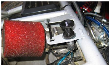
**Plunger Primer installed on Off Road Go Kart**
